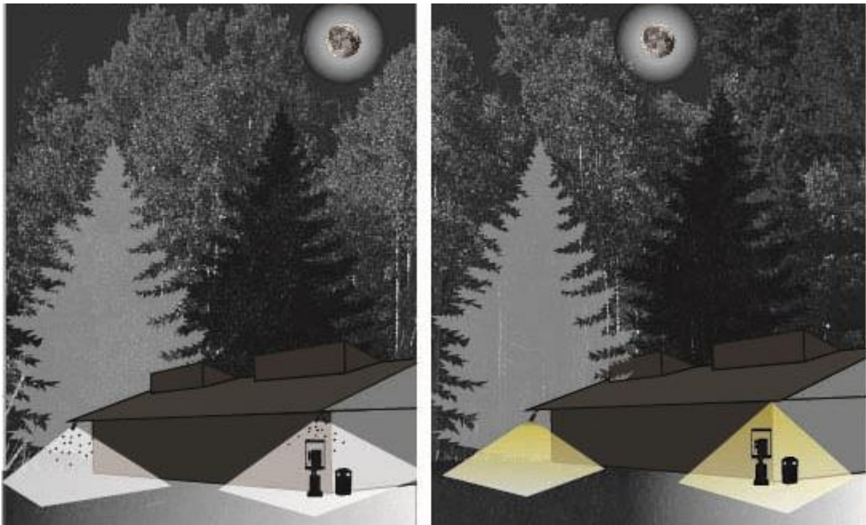
Figure 17. Yellow light that does not contain blue or ultraviolet wavelengths attracts far fewer insects.
